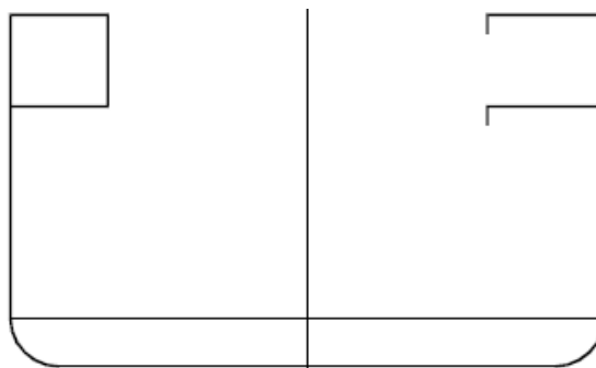
Figure 1.2: Container ship of single side skin construction
