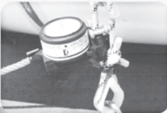
Correctly mounted Hydrostatic Release Unit (HRU) on an inflatable liferaft
