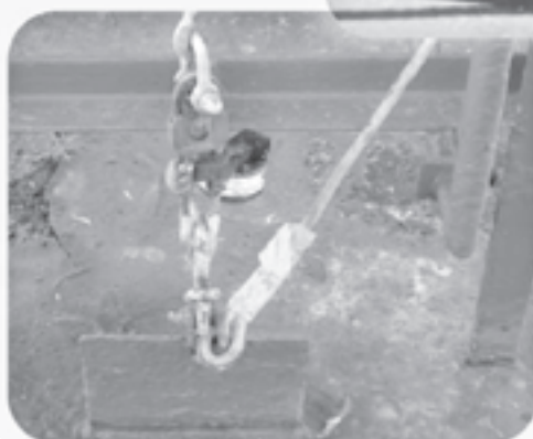
Incorrectly mounted HRU on an inflatable liferaft. The painter should be attached to the HRU
