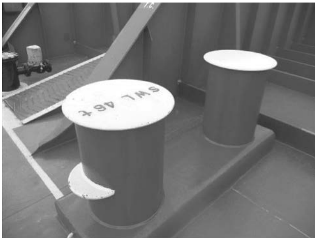
Mooring Bits on Oil Tankers – For securing Tug Lines, Fire Wires, and Mooring ropes / wires from other vessels during STS operations
