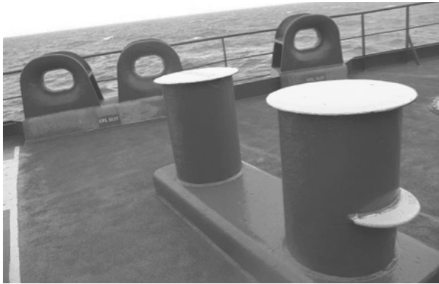
Mooring Bits on Oil Tankers – For securing Tug Lines, Fire Wires, and Mooring ropes / wires from other vessels during STS operations
