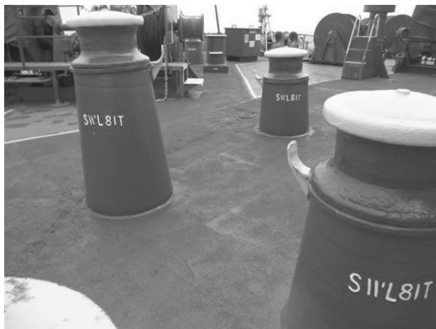
Pedestal Fairleads assist in guiding mooring lines for an appropriate lead
