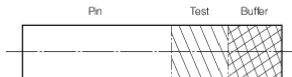
Figure 10. 4. 2: Buffer and test piece location for pins
