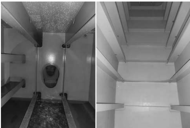
Figure 2. Interior of a Double Bottom (left) and Side ballast tank on a bulk carrier
