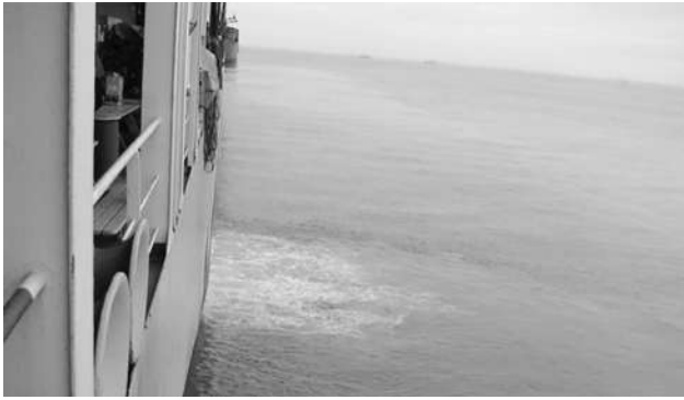
Figure 6. Discharge of ballast water below the water level from a container vessel
