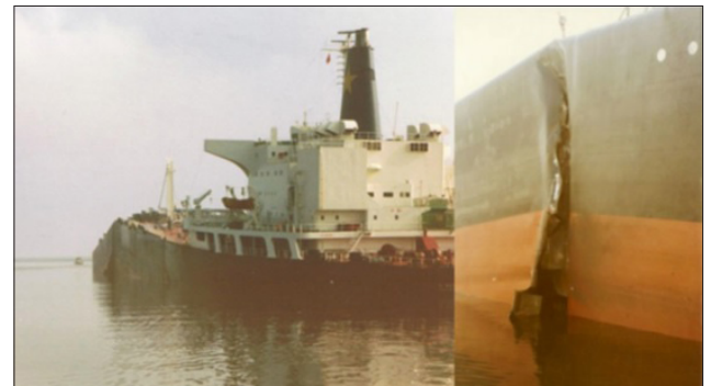
Figure 10. Vessel structure that failed because of overstress in hogging
