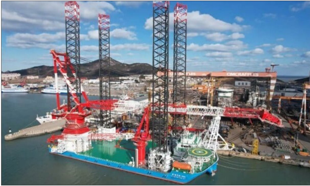
Wind turbine installation vessel designed to handle 20 MW and larger turbines
